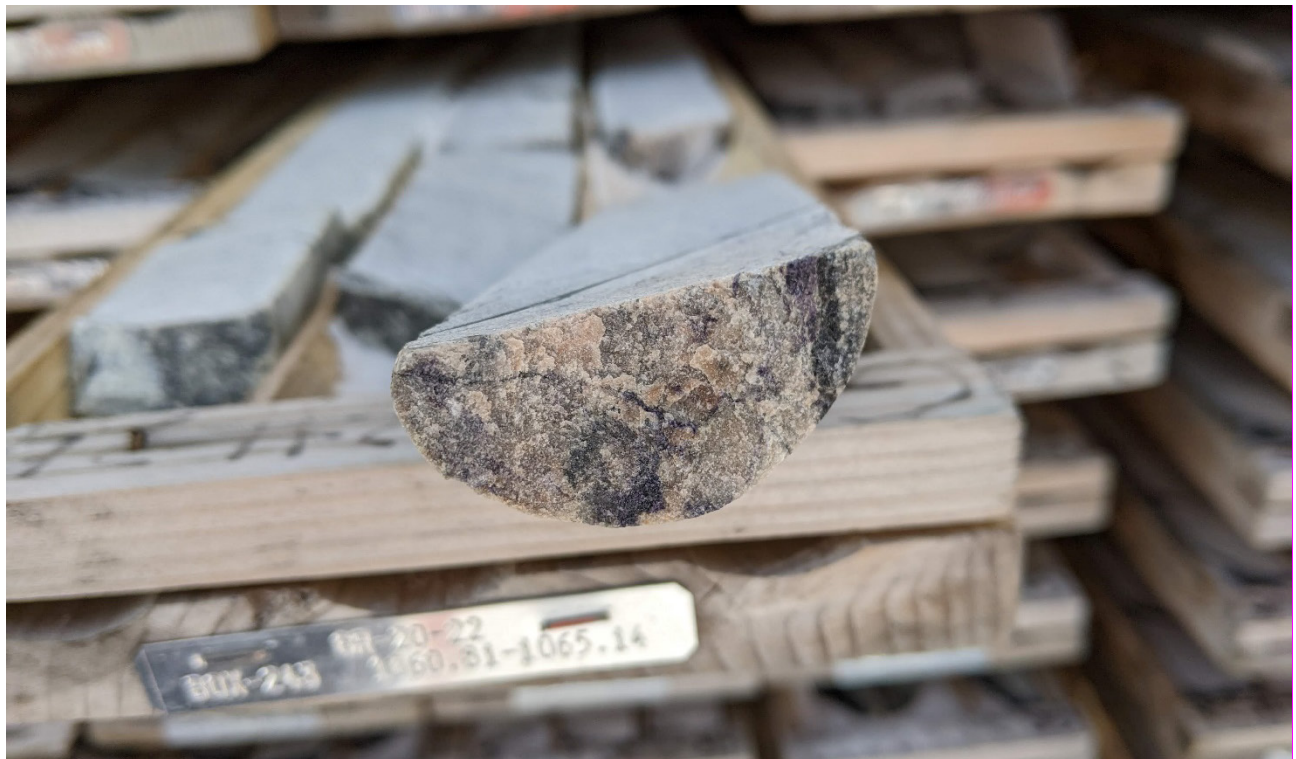
Figure 11-11 GR-20-22 from 1060 to 1065 m with Purple Mineral as Fracture Filling
