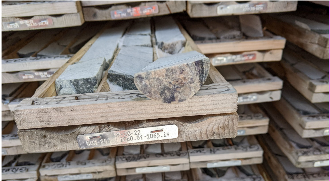
Figure 11-10 GR-20-22 from 1060 to 1065 m with Purple Mineral as Fracture Filling
