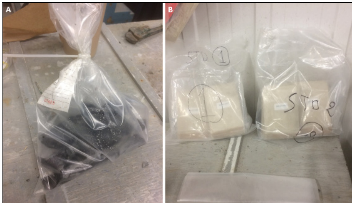
Figure 10-2 A) Sample in Plastic Bag with Tag; B) Two Standards used during the Drilling Program
