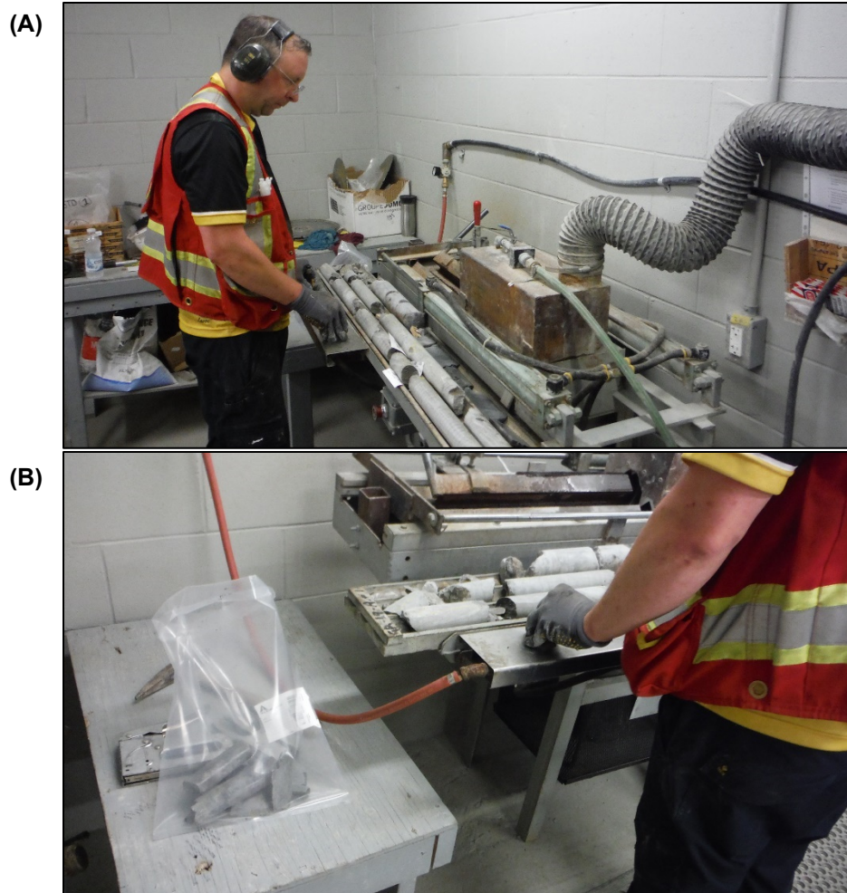
Figure 10-7 A) Core Samples cut in Half Using a Cutting Saw; B) Sample in Plastic Bag with Tag
