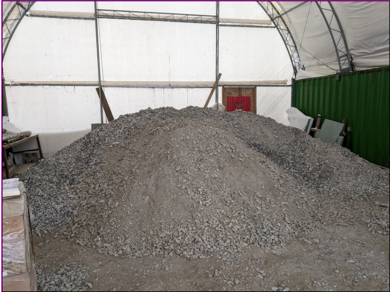
Figure 8-9 Bulk Material stored in a Shelter
